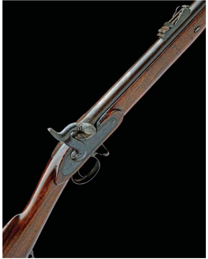
512 GEORGE GIBBS, BRISTOL A .577 PERCUSSION VOLUNTEER RIFLE IN THE MINIE STYLE, no visible serial number , circa 1860, with round 33 1/2in. barrel rifled in three grooves, bayonet bar at muzzle, block and blade fore-sight, elevating ladder rear-sight graduated to 1000yds., the breech-end of barrel signed 'GEORGE GIBBS, 29 CORN ST. BRISTOL' (rubbed), borderline engraved top-tang, borderline engraved lock signed 'GEORGE GIBBS' on the bar, military style hammer, walnut three-quarter stock with iron furniture, two cross-keys retaining the barrel, three swivels and jag-ended iron ramrod £600-800
